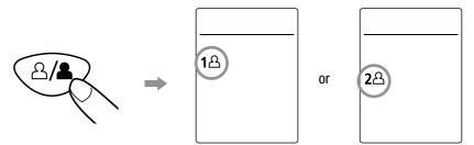
After a memory zone is selected, press th 0 button to reset the monitor so it can start measurement in the chosen memory zone.
